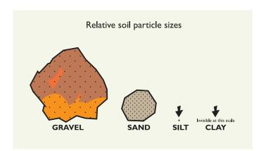
Soil is classified depending on its particle size, as shown in the illustration above. In gravelly soil, more than half the grains are pieces or rock that are larger than 4.5mm. If the grains are smaller, we call it sand. If the particles are so small that they are difficult to see, we call it silt. Clay is made of the tiniest rock particles.
